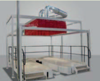
Special suction hood with lamellas at a robotic suction system
